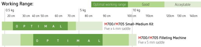
Optimal working range pr. machine & kits-size: White fish and Salmon measured in cm. with head
